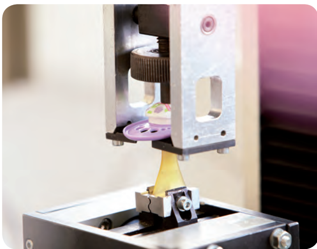
Quality test: MAM pacifier tensile strength
