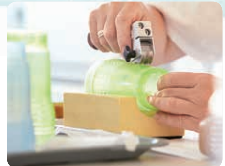
Bottles and soothers are thoroughly tested before they go on sale – they are stretched (above) and tested for durability and surface adhesion of the printing (below).
